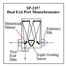
Figure 3. Includes micrometer controlled dual exit slits (90° & 180°). and motorized mirror for rapid, computer-controlled exit slit selection, rapid, computer-controlled exit
